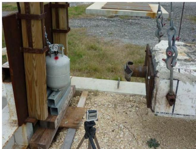
*Figure 13 CYL-1 Cylinder Prior to Testing.
