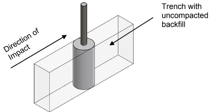
*Figure3 Unrestrained Bollard Installation*
