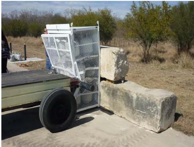
*Figure 10 SC-1 Cabinet Following Testing*
