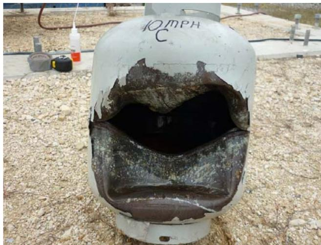
*Figure 15 CYL-7 Cylinder Following Testing*
