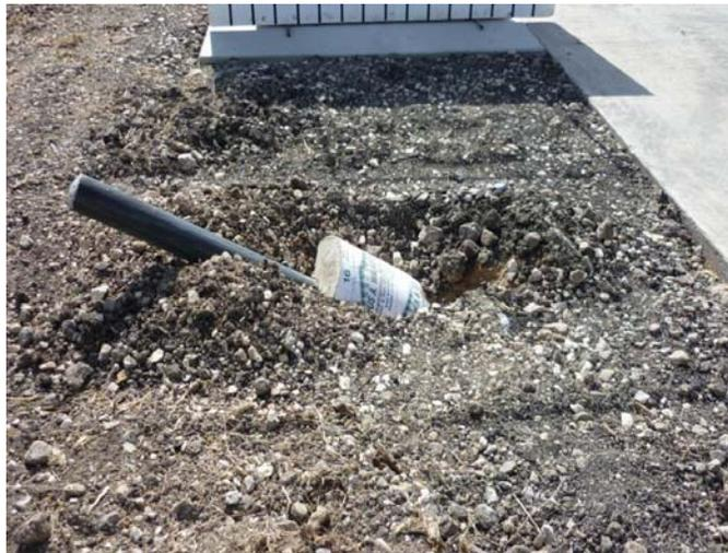
*Figure 5 URB-1 Bollard Following Testing*
